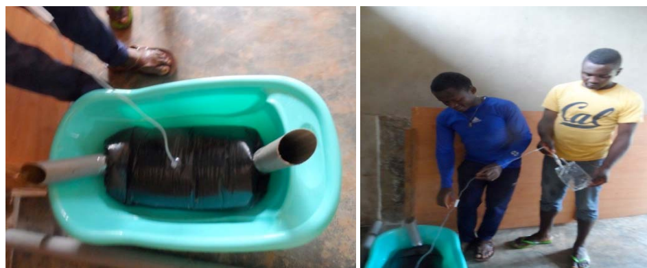
Plate 1: The anaerobic digester.
